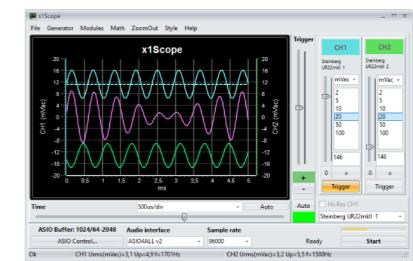
With x1Scope and a standard audio interface, you get a powerful oscilloscope with many additional functions. External USB audio interfaces with input gain controls for the 2 input channels are best suited.
