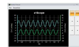
You can view saved diagrams from the oscilloscope, FFT module, YT module, and XY module later using Active Viewer. You can zoom in on the graphic using mouse gestures, hide individual channels, or move them horizontally using the arrow keys.
