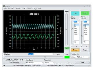
The module displays graphically the measured AC signal from the two audio interface inputs. Use the time base to set the scale for the x-axis and the voltage range to set the scale for the y-axis.
