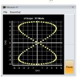
The XY module displays Lissajous figures. These are graphs created by the superposition of two harmonic oscillations at right angles to each other. The shape of the figures allows precise conclusions to be drawn about the frequency and phase of the two voltages.
