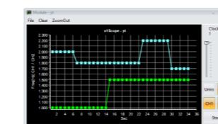
The “yt-Logger” module cyclically acquires the measured values from CH1 and/or CH2 (amplitude or frequency) and adds them to the measurement curve of the data logger. The clock rate starts at 1 second.
