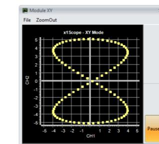
The XY module displays Lissajous figures. These are graphs created by the superposition of two harmonic oscillations at right angles to each other. The shape of the figures allows precise conclusions to be drawn about the frequency and phase of the two voltages.
