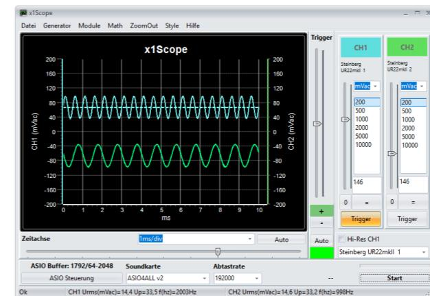
The module displays graphically the measured AC signal from the two audio interface inputs. Use the time base to set the scale for the x-axis and the voltage range to set the scale for the y-axis.
