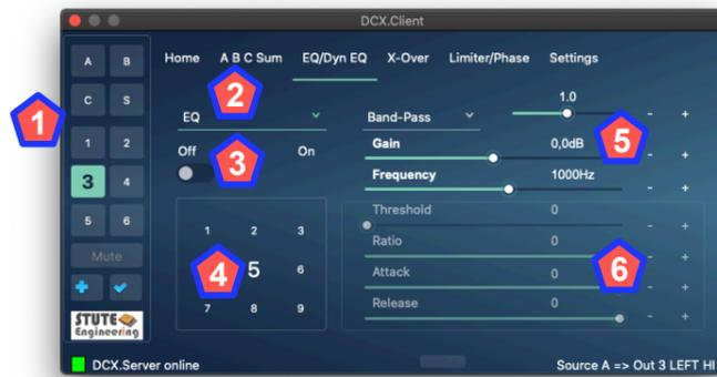
Control the 9 channel equalizer and dynamic equalizer for the inputs and outputs.
