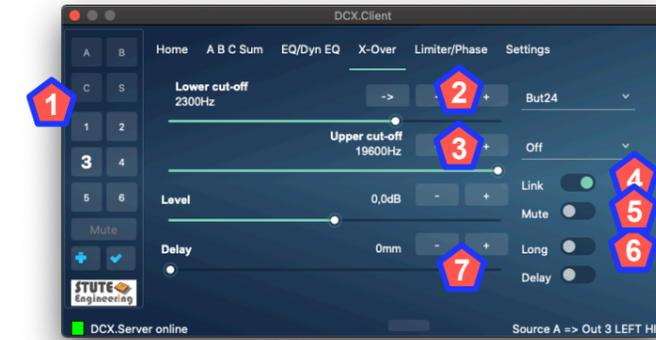
Control the cut-off frequencies, filter types and delays for the outputs 1 to 6.
