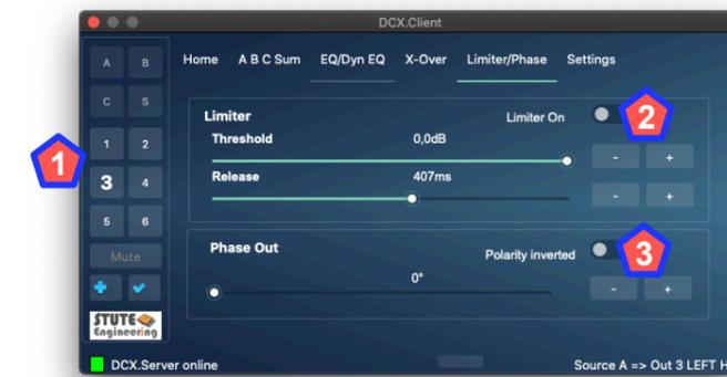
Adjust the limiter and phase settings for the output 1 to 6.
