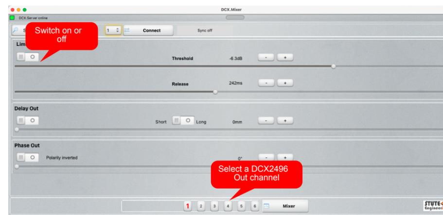
Control of "Limiter", "Delay" and "Phase" per output channel 1..6.
