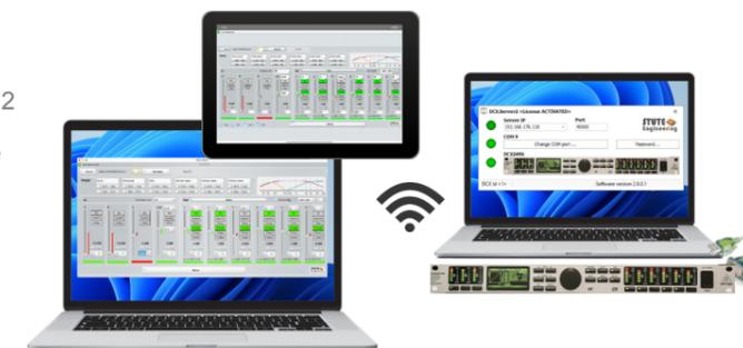
**Mode "Direct":** Control the DCX2496 with a single PC, e.g. prepare the DCX2496 settings in the studio. "DCX.Mixer / DCX.Client" and "DCX.Server" are installed at the same PC.
