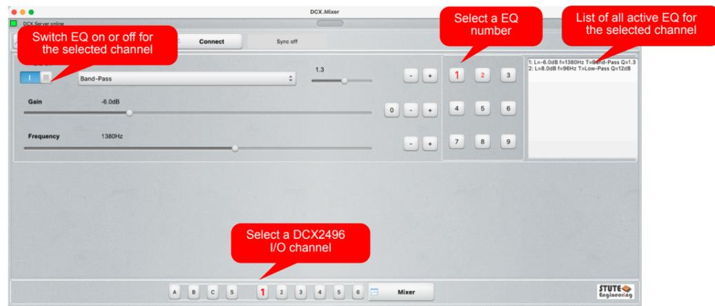
Control the 9 equalizer for each input and output channel.
